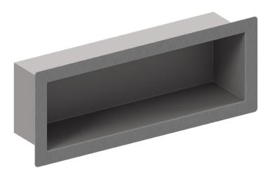
Metcraft's A811 ligature resistant shelf is fabricated from 14-gauge type 304 stainless steel. The box is mounted using two nuts welded on the rear of the shelf. Mounting this shelf requires a cutout measuring 16.15" x 5.15" and access to the rear side of the mounting wall.
