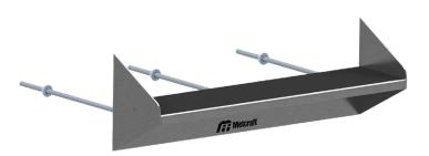
Metcraft's A731 ligature resistant shelf is fabricated from 14-gauge type 304 stainless steel. The box is mounted using three nuts welded on the rear of the shelf. Mounting this shelf requires three core drilled holes to allow anchors to pass through into the chase.
